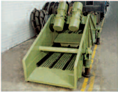
Vibratory screening machines
