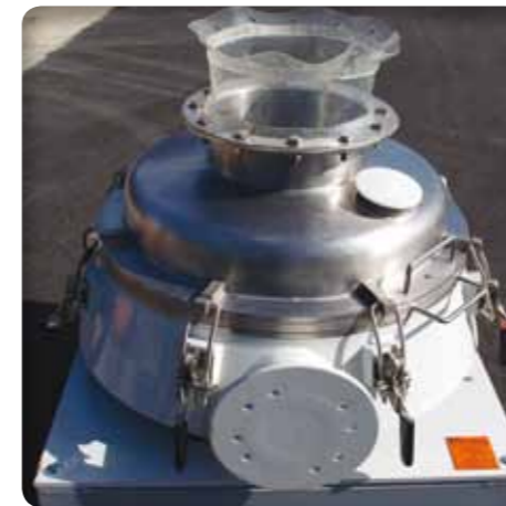
Entire vibratory sieve with flexible connection spout
