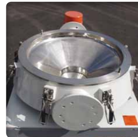
Vibratory sieve without mesh screen
