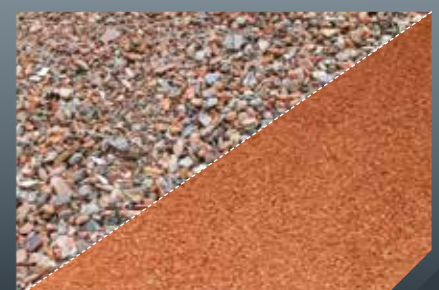
Screened C&D waste fractions
