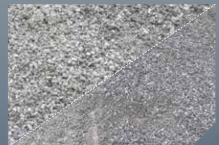
Screened asphalt fractions
