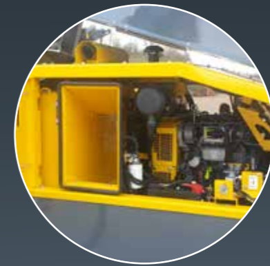
Wide access engine compartment doors Provide perfect access for service and maintenance of engine and hydraulics.
